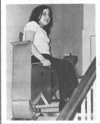
and does not interfere with the normal use of the stairs. This particular design can be plugged into an ordinary power plug; others have a small electric motor which is usually housed in the cupboard under the stairs. The lifts are operated by depressing a button, release of which stops the lift. They stop automatically when they reach the top or bottom of the stairs and carry up to 20-22 stones and all have built-in automatic safety devices.
